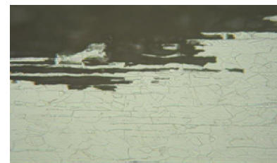
Figure. 5 : SX-6 macro and microstructure at 500x micro photo welding location corrosion area
